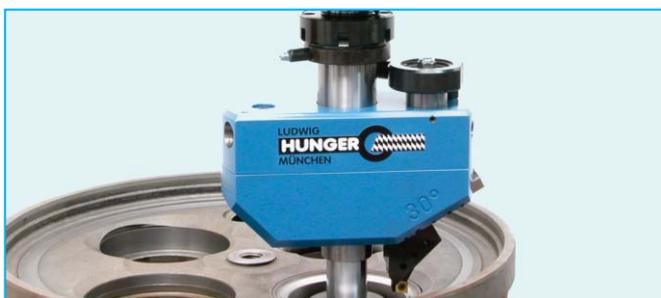
**UDM4E-VD Valve Seat Refacing Machine**
