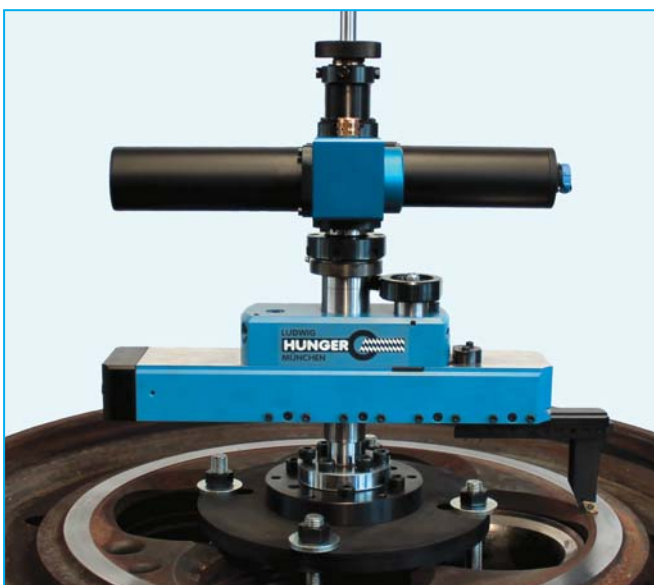
Face Turning Sealing Surface
