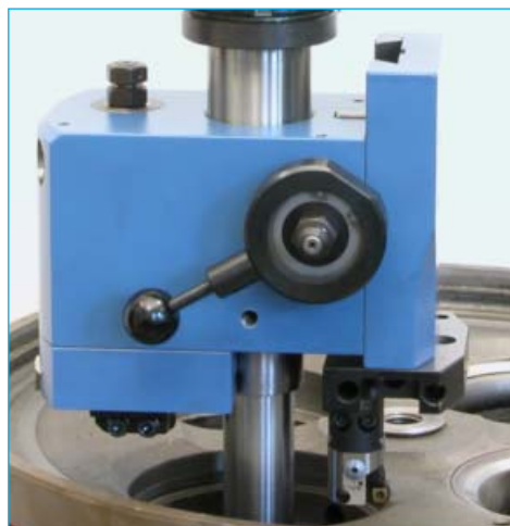
Counterboring Seat Ring Pocket
