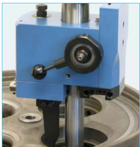
Refacing Bottom of Seat Ring Pocket
